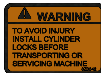
8Z0342 DECAL INSTALL CYLINDER LOCKS
