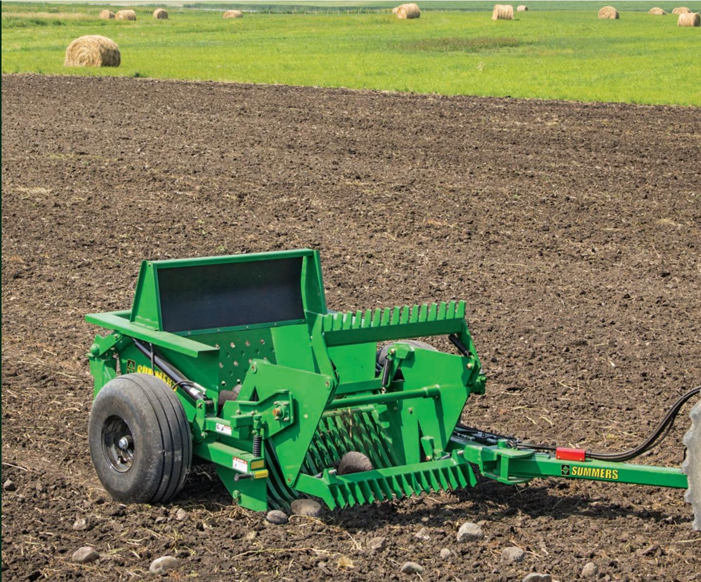
When it comes to continuous rock pickers, tough isn't good enough. It needs to be Field Tested Tough if you want something that holds up to years of abuse. Only Summers incorporates as many heavy-duty features, such as planetary hydraulic direct drive and reinforced batts, to keep you running, whether your rocks are two inches in diameter or 20.
