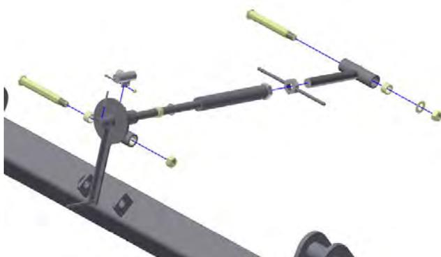
24. Install 8J5312 (T) onto side of poppet. Install 8J5710 from each end of poppet. Install 8J6020 on end of poppet.
