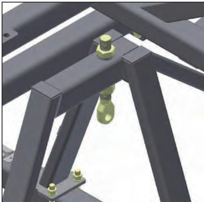
5. Insert eyebolts (8K1755) into each cylinder attach bracket. Tighten 1-1/2" nuts so the same amount of threads are above the top nut on all eyebolts. Ensure that cylinder attach holes are aligned when eyebolts are tightened.
