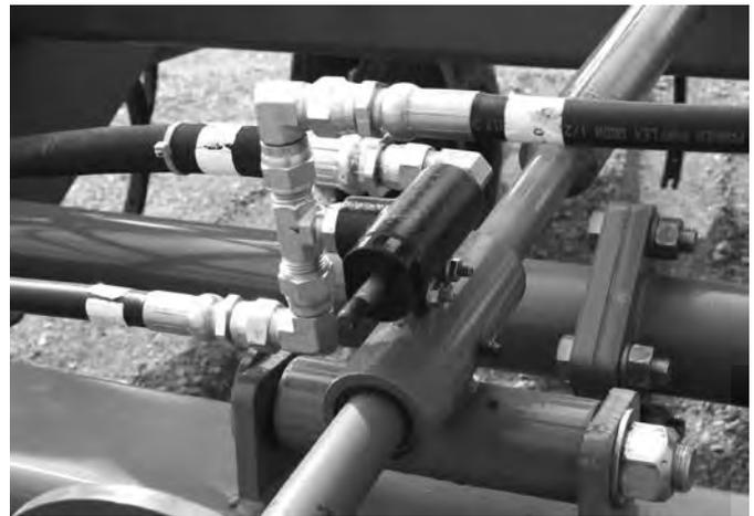
20. Install 8J6020 into base and rod ends of 8T1045, 8T1040B, 8T1037 cylinders. Hang cylinders according to layout.
