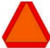
SMV emblems are only attached to vehicles traveling slower than 25 mph (40 km/hr). The most hazardous conditions to drive in are a daybreak and dusk. The use of a pilot car is recommended.
