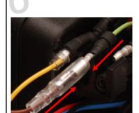
Connect the **BROWN** cable from the Lodar loom to the **LIGHT GREEN CABLE (SGND)** on the Honda engine.
