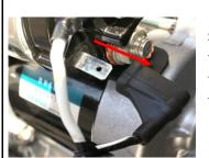
Remove the **BLACK AND WHITE SOLENOID+** signal cable from the Honda engine. This can be found on **FUNCTION 3** with in the engine photo on page 1.
