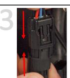
Connect the **MALE** side of the Lodar loom to the **FEMALE** connector on the Honda engine. It will only mate in one position.
