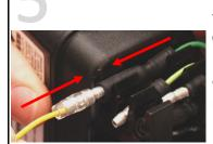
Mate the YELLOW cable from the Lodar loom to the DARK GREEN GABLE (SW2) on the Honda engine. This can be seen on FUNCTION 1 in the engine photo on page one.
