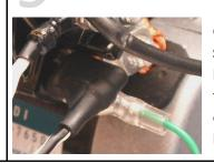
Connect the **BLACK AND WHITE SOLENOID+ CABLE** by piggy backing on to the **GREEN CABLE**from the Lodar loom. This will enable control via the ignition key switch.
