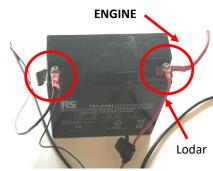
The Lodar and the engine can be connected to the battery as shown.
