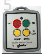
The **STOP** (**OFF**) button on the **TRANSMITTER** can be pushed to turn off the engine, all the lights on the **RECEIVER**, except the power light, will turn off to indicate that the ignition has been deactivated. The engine will **NOT** turn off using the transmitter if the key is not set to the off position. The engine can not be restarted for a period of **THREE** seconds, this is a safety feature and **CAN NOT** be disabled.
