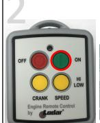
Upon pushing **SET (ON)** on the **TRANSMITTER**, the following lights will illuminate on the **RECEIVER** to indicate the ignition is on. A relay will simultaneously energise upon setting the receiver. If no sound is apparent, please contact your dealer. A safety feature has been placed on **SET** to prevent the user from reactivating the
