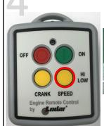
The **F2 (HI LOW SPEED)** function will dictate the engine speed. A successful push will latch the function to **INCREASE** the engine speed and turn on the respective lights on the **RECEIVER.** A relay will energise at this point. If no sound is apparent upon pushing F2, then please contact your dealer. There is no time out require-
