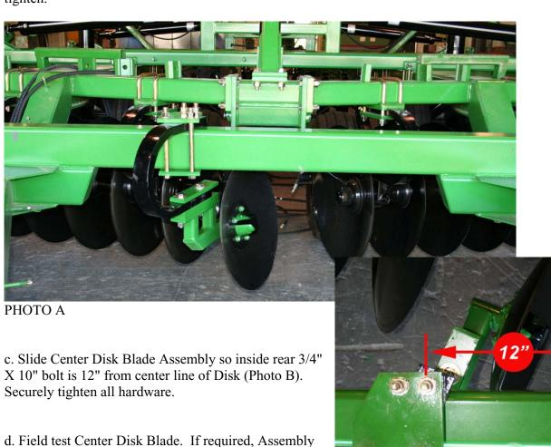
d. Field test Center Disk Blade. If required, Assembly can be adjusted side to side by loosening 3/4" X 10 bolts, reposition and retighten hardware. Depth of the Center Disk Blade can be adjusted by installing or removing 8K4930 flats.
