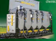
Along with speeding up sprayer fill times, the Spray Fill Xpress has a unique batching process that allows farmers to precisely measure each chemical before individually adding them to the water stream.
