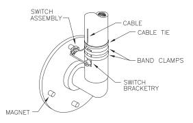
**Note:** The switch assembly does not need to pivot with the wheel.
