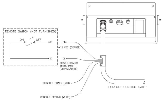
An optional remote switch may be installed if the console is mounted in a location that is not easily accessible. A remote switch may include a foot switch or a toggle switch on the joystick. To utilize the remote switch, the master switch on the console must be turned off. The master switch on the console can be used again once the remote switch is turned off. Refer to the figure above to install the optional remote switch.
