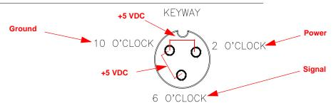
**Note:** If a +5 VDC voltage reading is not present, disconnect the flow sensor cable. If the speed reading is restored, refer to the Testing Flow Meter Cables section on page 44 to test the flow meter cables.
