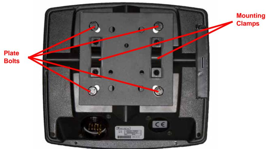
**Note:** The mounting clamps are designed to secure the console to a 1" dia. [2.54 cm] monitor bar or post.
