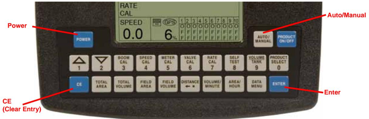
**Note:** The initial programming sequence must be completed before the SCS console can be operated normally. Calibration values must also be programmed on the calibration screens accessed through keys 3 through 7.
