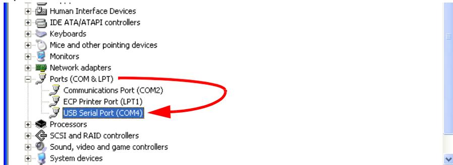
8. Double click on “USB Serial Port” to display the “USB Serial Port Properties” window.
