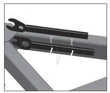
22. Place adjustment wrenches on clevis pins found on left hand of hitch. Retain with hair pin clips.
