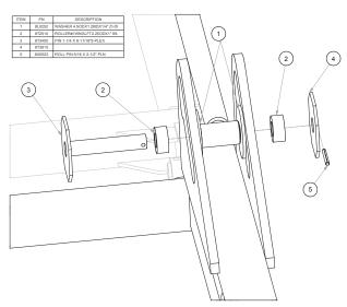
9. Connect rod end of 5" x 36" cylinders to part 1 wing. Install wing lift pin, rollers and washers onto the wing and cylinder rod tube. Secure pin with 8T3810 washer and roll pin. The 8L0250 1/4" thick washers must slide freely inside wing flamecuts. The drawing below shows an end view of this connection. Grease rod end tube on 5" x 36" cylinders before lifting wings. Also grease part 2 wing pivot pins.
