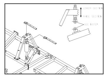
5. Leveling the chisel plow from side to side. Stop the tractor with the machine still in the ground. Check the depth of tillage on the left wing, center, and right wing. If leveling is necessary, use wrenches provided to adjust the eyebolts on the cylinder attachments located at the rear of the machine.
