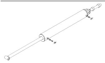
3. Install hoses that supply base end of part 1 wing lift cylinders. Install 35" hose from one right hand port of the manifold block (A & B) to the base end of both front 5" x 36" cylinders. Connect base end of rear 5" x 36" cylinders to front cylinders with 70" hoses.
