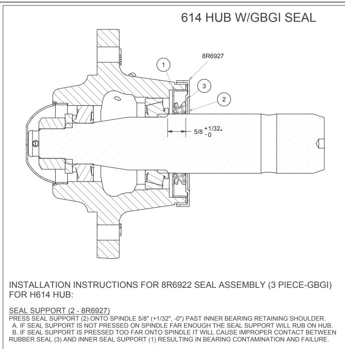
NOTE: APPLY THIN LAYER OF GREASE TO COUNTERFACE (1) SURFACE AT TIME OF SEAL INSTALLATION.
