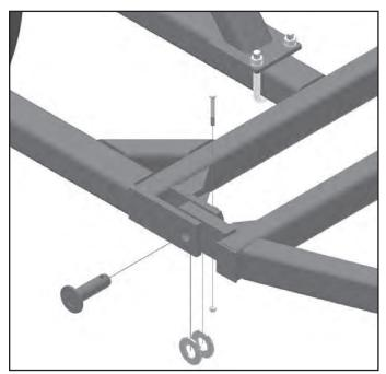
1. Attach wing to center section with pins, washers, bolts and locknuts.
