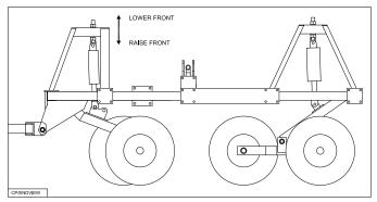
The front center lift arm has two cylinder attach locations. If chisel plow has a full set of mounted harrows or if rear of machine is low in transport position, use rear cylinder attach hole. Connecting front center cylinder to rear hole will lower front of chisel plow in transport position.
