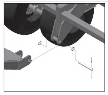
15. Attach hitch to center with 1-1/2" x 10-5/8" pins.
