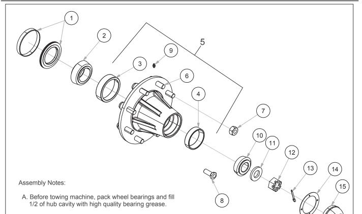
B. Tighten axle nut to 45 ft.-lbs., loosen nut until first slot is aligned with hole in axle, install cotter pin and bend to retain.
