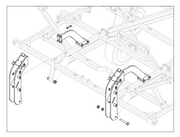
15. Install two 8CC6026 and two 8CC6022 onto 8T3950 with pins. Secure pins with roll pins. Connect the two 8CC6026 together using 7/8" x 3" bolts, lockwashers and nuts.
