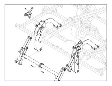
16. Install 8CC6000B (pivot tube) onto 8CC6022
