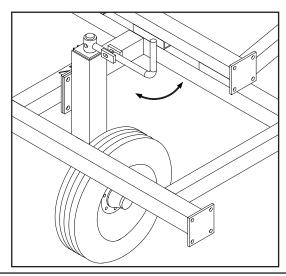
**IMPORTANT!** Gauge wheels are only intended to stabilize the machine. They should not be used to support entire weight of the wings. Tough soil conditions may create "suction" on the front of the chisel plow. As long as the machine is not operated beyond the trip assembly limit (see page 4-3), the gauge wheels are being used properly. Failure to follow these guidelines may result in machine damage.
