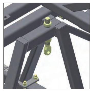
Insert eyebolts (8K1755) into each cylinder attach bracket. Tighten 1-1/2" nuts so the same amount of threads are above the top nut on all eyebolts. Ensure that cylinder attach holes are aligned when eyebolts are tightened.
