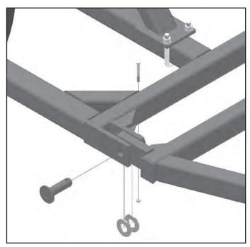
1. Attach wing to center section with pins, washers, bolts and locknuts.
