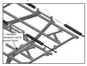
12. Insert 1-1/2" x 10-3/8" eyebolts into wing lift cylinder attach base. Leave 1-1/2" nuts loose, they
