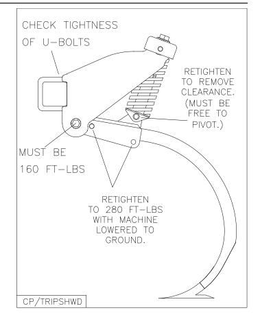
6. Check tightness of all hardware. Pay special attention to hitch bolts and all pivot retaining bolts.
