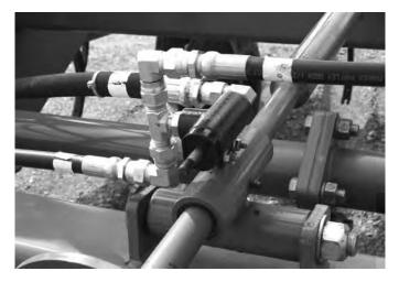
26. Install 8J5310 and 8J5710 along center of machine. Join 8N4198 and 8N4160 using one 8J5510 and attach to 8J5710. Run other end to front of machine. Join two 8N4216s using one 8J5110 to run off each side of 8J5310. Attach other end of this to rod ends of 8T1037.
