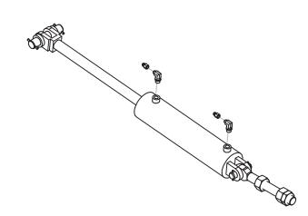
7. Connect two 330" hoses to front side of manifold block (Z). Route these hoses to front of hitch along same path as depth control hoses. Leave slack by the hitch pivot. Install 3/4" ORB x 6 JIC(M) adapters and ISO tips onto ends of 330" hoses. Install yellow nylon ties by tips and closest cylinder to identify Wing Lift circuit. Use nylon ties to hold hoses away from pinch points.
