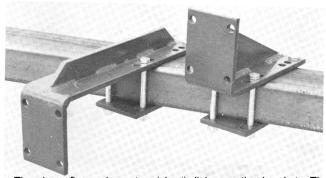
1a. The above figure shows two (short) disk mounting brackets. The universal model on the right is designed to be mounted on top of the frame with the mounting plate extending up. The high clearance model on the left is designed to be mounted on top of the frame with the mounting plate extending down. The high clearance model is also longer to provide clearance for disk scraper assemblies.
