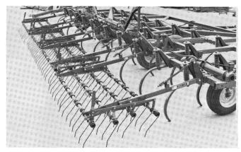
1a. The above 29' JD1610 chisel plow is shown with a 4 bar mounted harrow using M74 carrier arms. Two 7' sections were used in the center and one 8' section was used on each wing. An optional method is to use one 14' section in the center with 3 carrier arms. Wing section sizes will vary with the width of the chisel plow.
