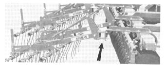
2a. The above figure shows a short and a long high clearance disk bracket used to mount a 7' section. When carrier arms are spaced 2 teeth apart on high clearance brackets or 3 teeth apart on universal brackets, the carrier arm bolts directly to the disk mounting bracket using the four 5/8 x 2" bolts supplied with the disk brackets.
