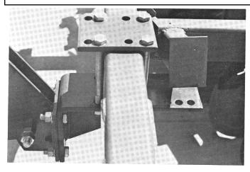
3a. Bracket #2 is a modified short universal disk bracket (PN 8H1546) that mounts to the disk main frame as shown above. Secure using a 1/2 x 5 x 6-1/8" mounting plate (PN 8H1340) and four 5/8 x 8" bolts.
