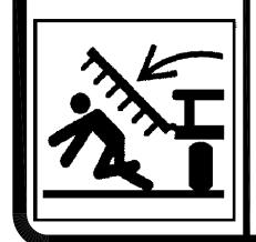
TO AVOID INJURY OR DEATH STAND CLEAR OF MACHINE WHEN WINGS ARE BEING RAISED AND LOWERED. MECHANICAL OR HYDRAULIC FAILURE CAN ALLOW WINGS TO FALL RAPIDLY.
