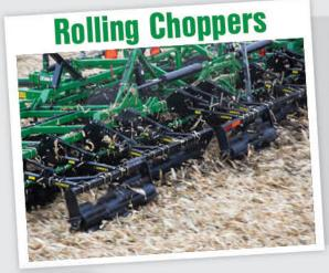
When it comes to primary tillage, breaking sod or grass, and extremely heavy residue management situations, a mounted rolling chopper excels.
