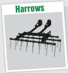
Harrows distribute residue and level soil. Summers mounted harrow models — available in 3- and 4-bar configurations — differ by tine diameter and length. In general, larger diameter and longer length result in more trash clearance and aggressiveness, whereas a smaller diameter and shorter length is less aggressive but leaves a better field finish.
