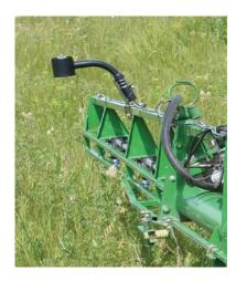
Optional Norac Boom Height Control maintains a constant boom height. Five sensor package is standard on Ultra Ultimate NT only.
