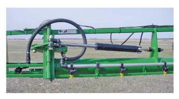
On both the Ultra and Ultimate NTs, a **Patented multifunction fold and breakaway system** is coupled with the breakaway protection designed into the hydraulic system. The nitrogen charged accumulator assists gravity to smoothly return the boom to field position after the obstruction is cleared.
