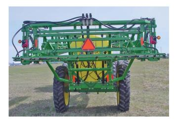
Telescoping axles provide extra stability in wide wheel settings. The standard cart with a standard axle has wheel adjustments of 88 - 132 in. using the standard 480/80R38 and optional 380/90R46 tires. The 380/90R46 tires permit spacing adjustments from 76 - 120 in. with the narrow axle. When utilizing a wide axle, wheel spacing can be adjusted from 109 - 152 in. with both tire sizes. The narrow cart sprayer with a
