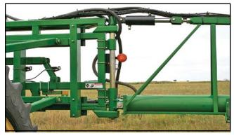
Separate Hydraulic **tip lift cylinders** allow the ends of each boom to be lifted to clear obstructions or to compensate for slopes and uneven field conditions.
