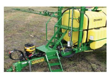
The spray system features corrosion resistant components and includes electric ball valves for left, right and center boom sections. An electric dual jet agitator, boom line strainers, 2" bottom fill, and boom drains are standard equipment. Agitator flow control and in-line strainer complete the system.
