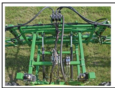
This top view of the boom suspension system depicts lift cylinders and accumulators.
