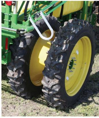
standard axle allows wheel adjustments from 60 - 89 in. and will accommodate 30 in. duals spaced at 60 and 120 in. The optional wide axle for this sprayer may be adjusted from 76 - 113 in. and will accommodate 20, 22 and 30 in. duals. The 20 in. duals can be set at 80 and 120 in.; the 22 in. duals (shown) can be set at 88 and 132 in.; and the 30 in. duals can be set at 60 and 120 in.
