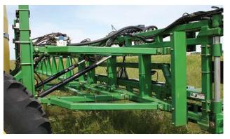
Rugged, parallel linkage helps maintain rigidity in boom lift system and maintains nozzle orientation to ground throughout all height settings.
