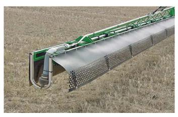
**Ultimate NT:** Flexible windscreens are optional on on boom sizes from 60-110 ft. and provide supplemental aid in reducing spray drift. **Windscreens are not available for the Ultra Ultimate NT.**
