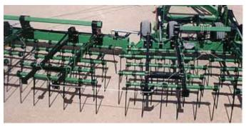
Standard *back-up* feature allows operator to back up with machine in field position in order to reach isolated areas and tight corners.
