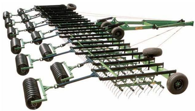
Built for high speed operation, the Harrow Packer is a proven tool for moisture conservation. Constructed of all-welded tube steel and engineered for field tough conditions, this unit can provide a one-pass seedbed without pulverizing the soil surface.
