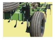
S-tine ranks are equipped with hydraulic cylinders to "roll" tines either partially or completely up. Partial retractions can be used for depth adjustment.
