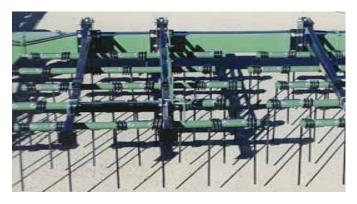
The **Summers** *exclusive* top mounted torsion bar pressure springs provide a streamlined design for optimum residue clearance.
