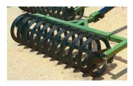
Packers are 1-3/4" square steel (130 lbs./ft.) coils. Units are mounted to conform to varying ground contours.
