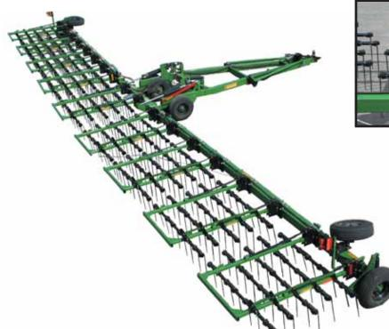
Featuring the new 1/2" dia. X 26" tooth with increased action for improved soil tilth and residue management.
