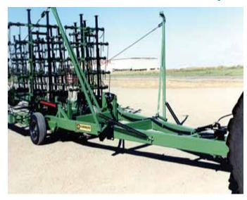
The drawbar is a massive  $8 \times 8$  in. square tube for maximum strength with 11 LRF x 15" tires (optional 31 x 13.5 on hitch) for necessary flotation.
