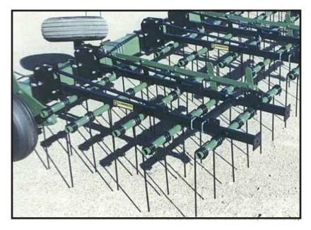
**Plus**, it can also be used for seedbed preparation, light tillage, granular incorporation, and to spread and break up residue after the combine.
