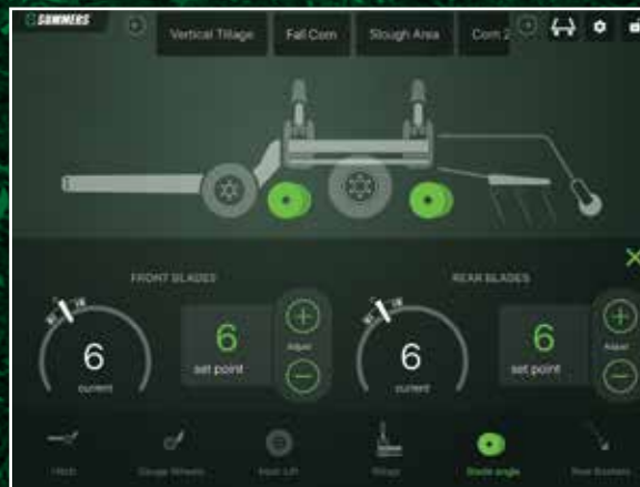
Hydraulically Adjust Front & Rear Blade Angles from 0 to 19 Degrees
