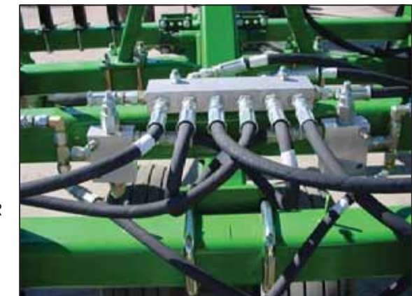
REAR VIEW MANIFOLD AND SEQUENCING VALVES
