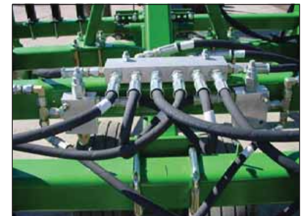
REAR VIEW MANIFOLD AND SEQUENCING VALVES
